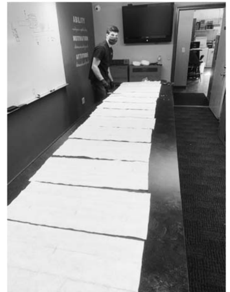
After the filters are dismantled, there is a lot of filter material - which is part of the reason why they are so effective filtering the air in a house. Pictured is 'T3' in the process of cutting the filters into smaller pieces— like the ones sent to you.
